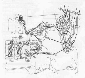
Press pushbutton and lift looper thread take-up to thread the machine easily.
